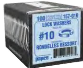
Papco® Lock Washers provide a locking spring action against the tendency of threaded assemblies loosening due to vibration. They are made to specifications of the Society of Automotive Engineers (S.A.E.) and the current ANSI B27.1 standard. They are supplied in Regular, for Grade 2 bolts and low load applications; Extra Duty for Grade 5 or 8 bolts and high load applications; and Hi-Collar for Socket Head Cap Screws.
